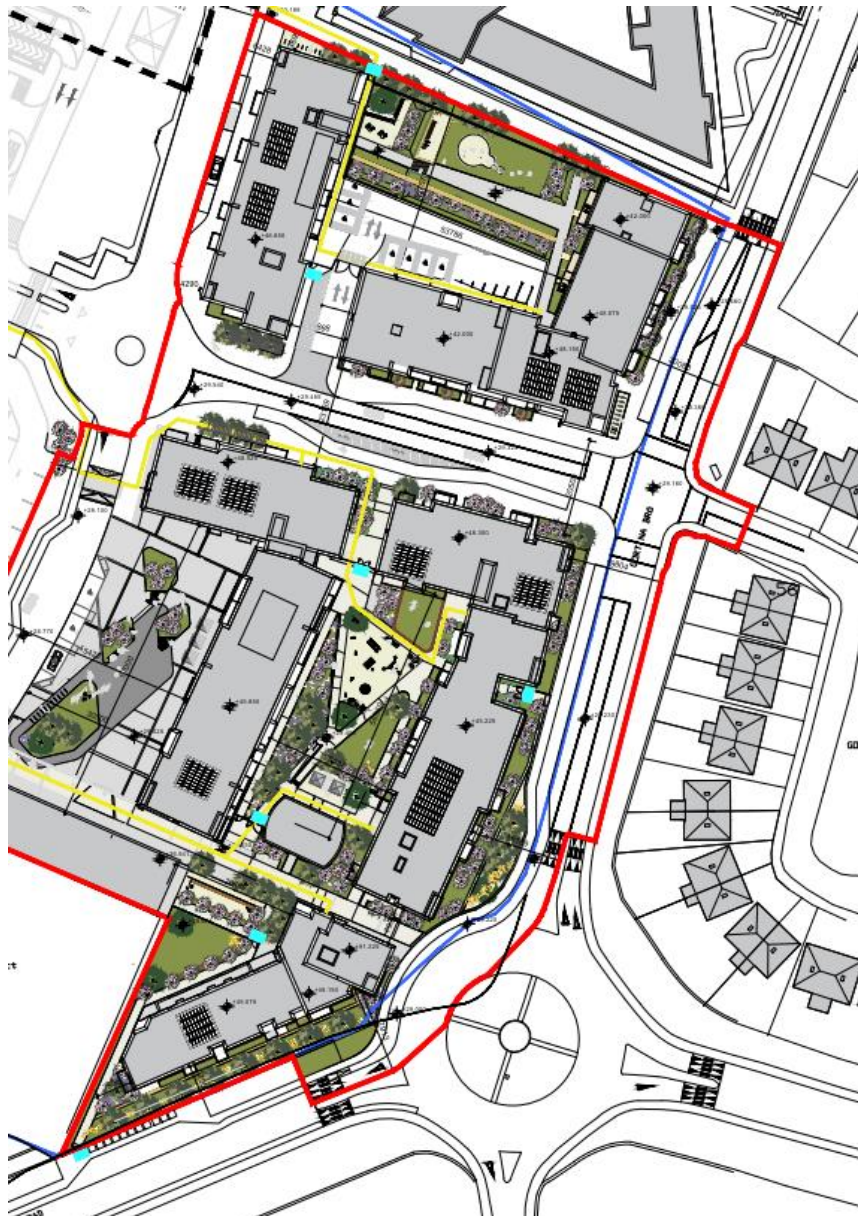
Fig 2 Location of controlled access gates (cyan) where residents shall have 24 hr access.
